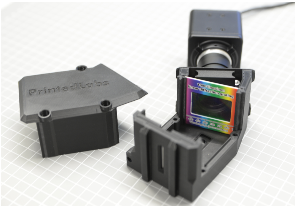
Figure 3: Assembled spectrometer and front cover
